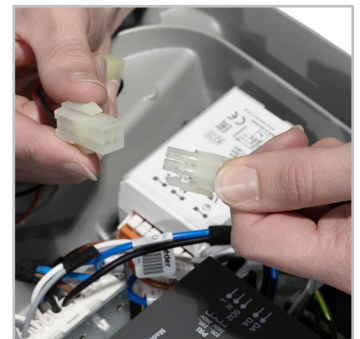
Poke-yoke connectors for easy, failure-proof integration into your TECEO 1 luminaires.
