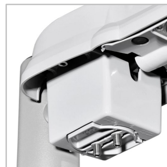
AXIA 3 EVO has a universal fixation part for spigots ranging from Ø32 to Ø76mm. It can be adjusted on site in 2.5° increments to provide precise lighting and optimise photometry.
