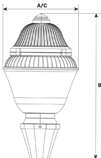
TEMPORE GEN2 | Post-top mounting onto 1/4" threaded spigot
